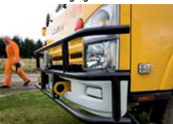
A bull-bar is a handy addition, along with ferry tie-downs that double as towing eyes.
